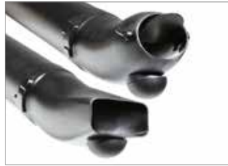
Two air delivery nozzles supplied as standard: rectangular/round section, both equipped with hemispherical support so the tube can rest on the ground on level terrain to reduce operator fatigue ( SA 9500 ).
